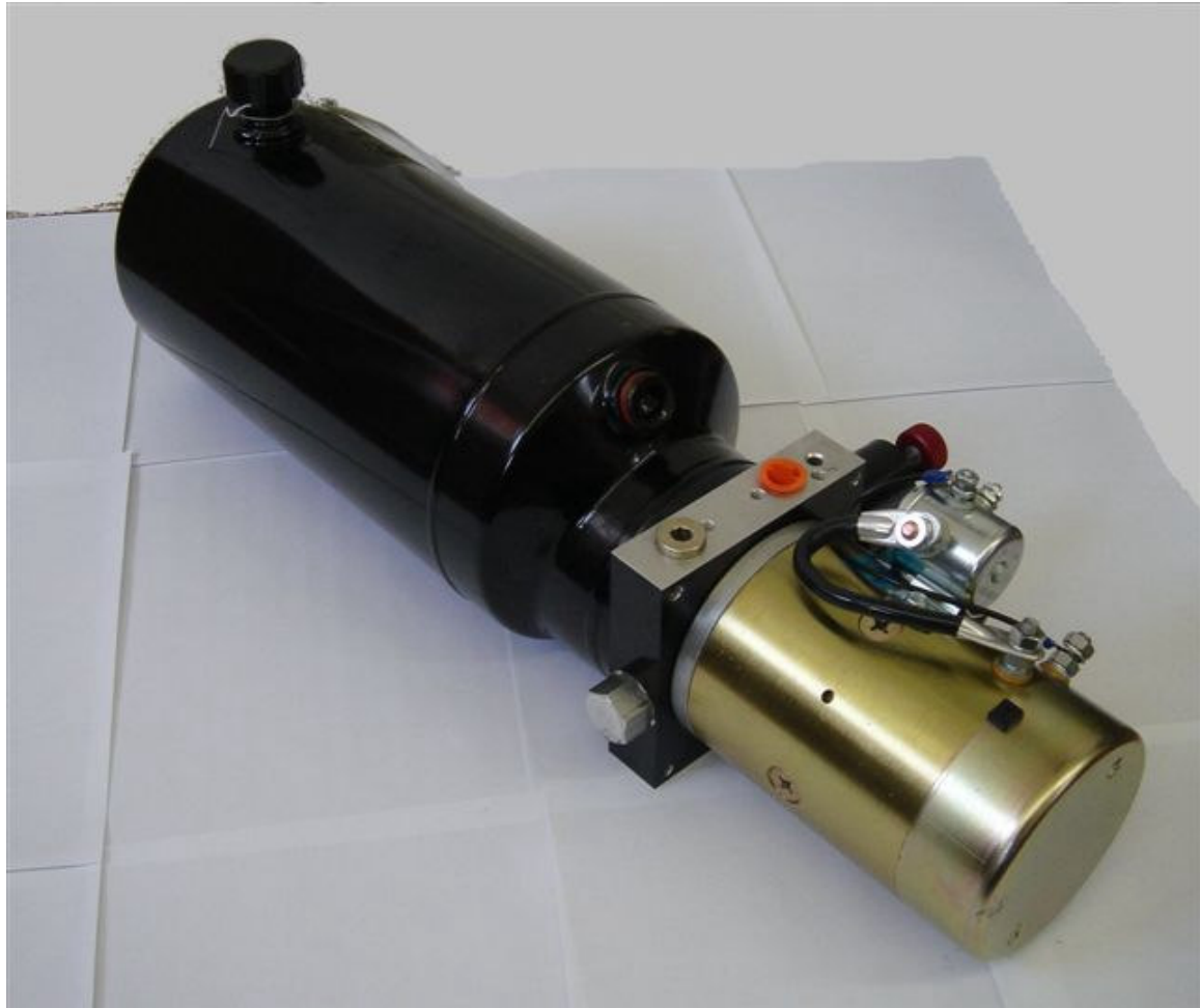
Figure 6.6 - Assembled hydraulic power pack
