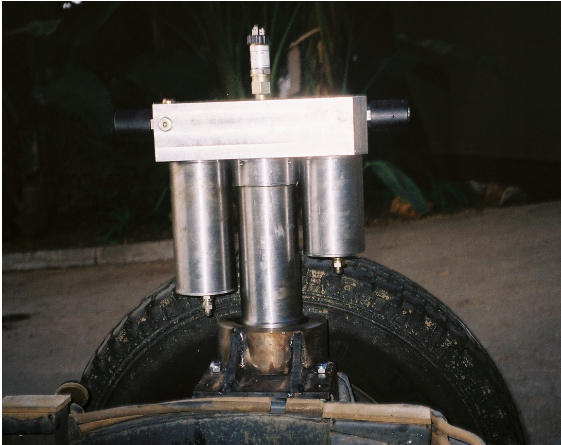
Figure 6.2 - Right rear suspension fitted to chassis – inside view
