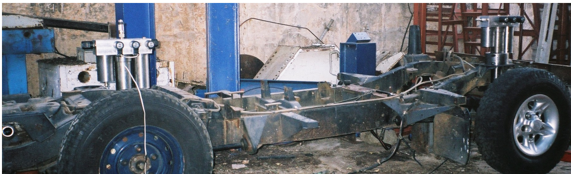
Figure 6.3 - Right front and right rear suspension fitted to chassis
