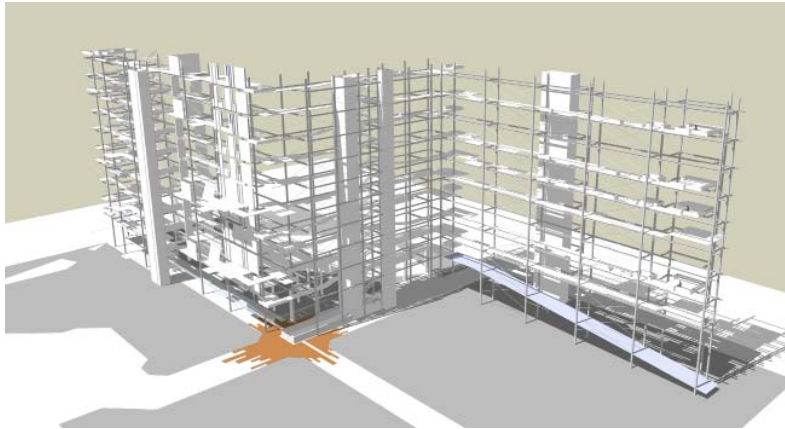
Fig. 89: Structural members have been re-sized and removed to aid the design of a permeable structure, allowing natural ventilation and light to penetrate the space (Author, 2010).
