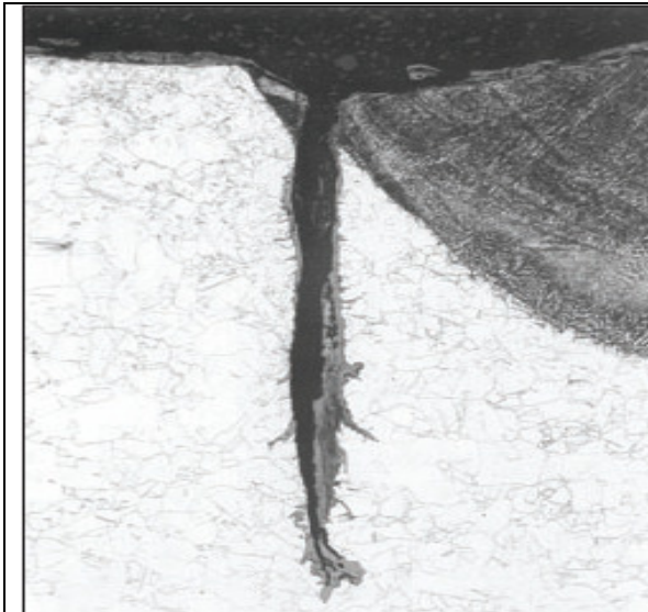
Figure 2.14 Corrosion fatigue adjacent to weld in 316 stainless steel pipeline [27]
