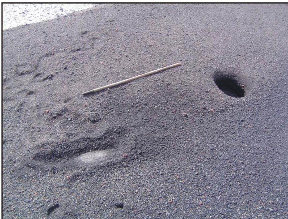
Figure 4.9: Excavations of ground in the interior of Marion Island at approximately 1000m a.s.l. in late austral summer (March 2005) indicate that within a very small area the ground can remain ice-cemented (left of centre) or provide no evidence of frozen ground (right of centre). Rod is 1.2m in length (March 2005).
