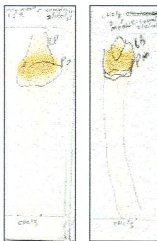
Fig. 35 TLC of chloroform fraction using different ratios of chloroform and methanol combination as solvent systems. From left to right: ratios 1:2, 2:1. Lines represent fluorescing compounds.
