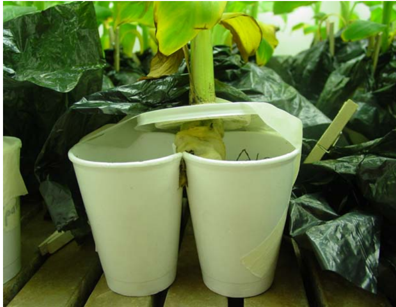
Figure 1: Roots of banana were split into two parts, and each half of the roots was planted in a 250-ml cup in a split-root experiment. The cups were filled with 150 ml water to prevent overflow of water into the other cup. Strips of sponge were wrapped around the stems to ensure that the lids did not damage the stems. The exposed stems were covered with wet cotton wool, and the cup system was enclosed in a black plastic bag to prevent the roots from drying out.
