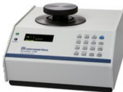
Figure 32. Typical Micromeritics AccuPyc II 1340 gas pycnometer
