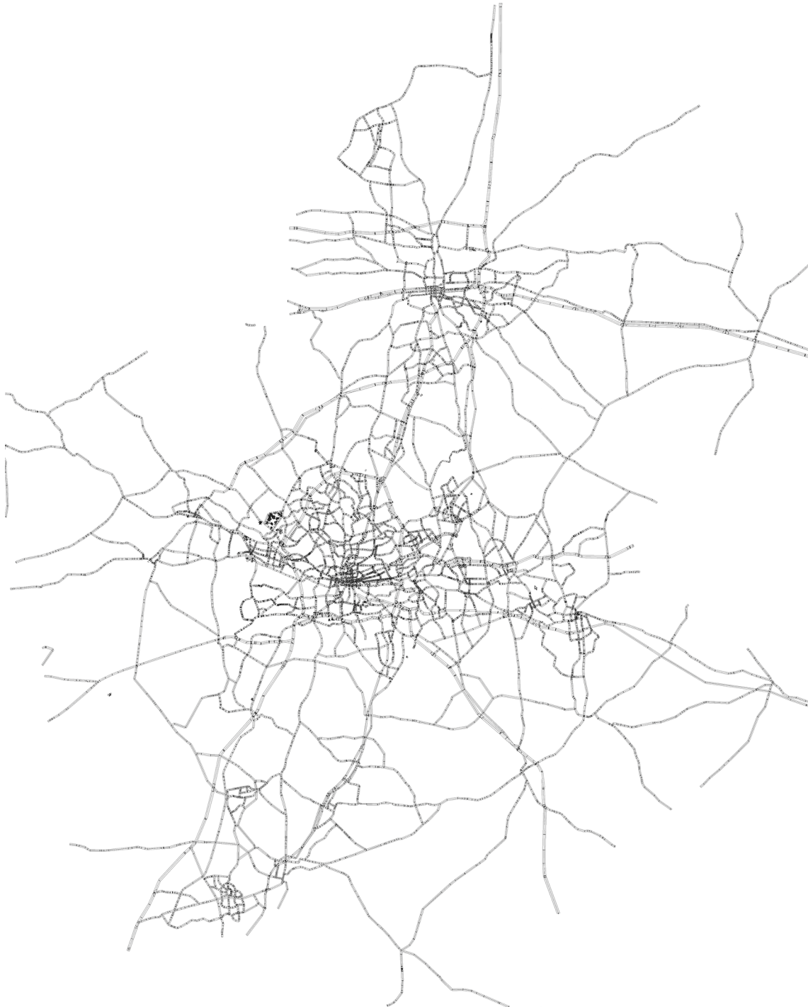
Figure 3.3: Reduced or small network representation derived from GIS shapefile, depicting only main road and higher level network links.
