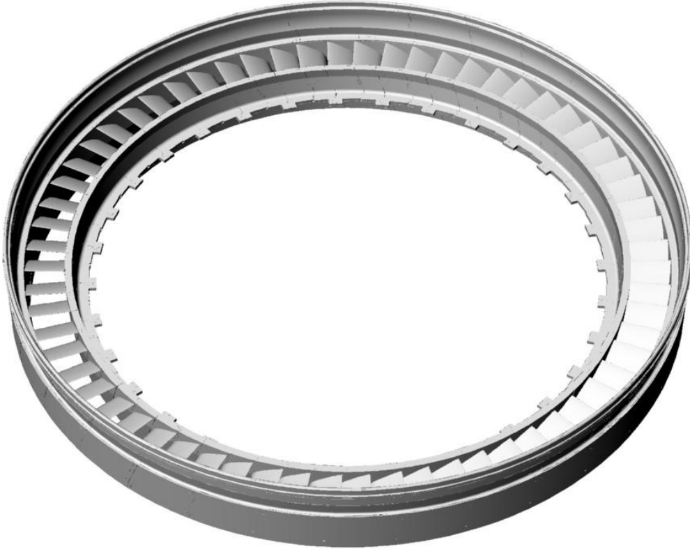
Fig. 2.5 T56 NGV 60-blade assembly
