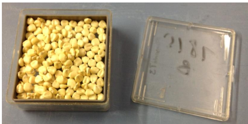
Figure 11: Maize seeds placed on a wire mesh in a container used for the accelerated ageing test.
