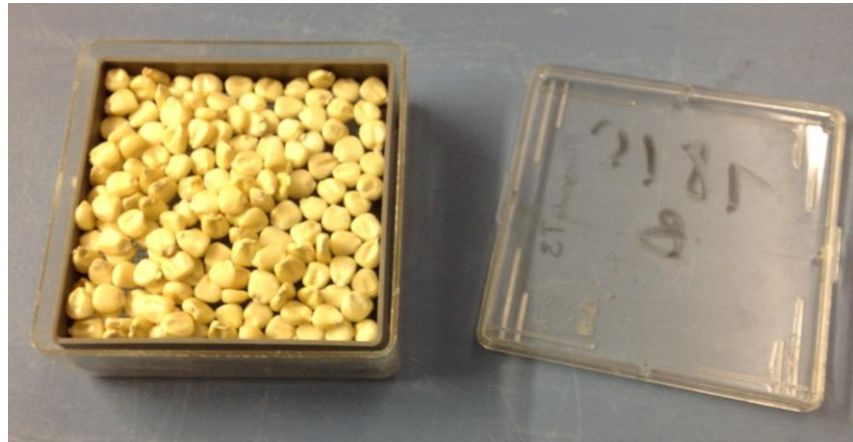
Figure 13: Maize seed placed on a metal grid in an accelerated ageing container in preparation for undergoing an accelerated ageing test.
