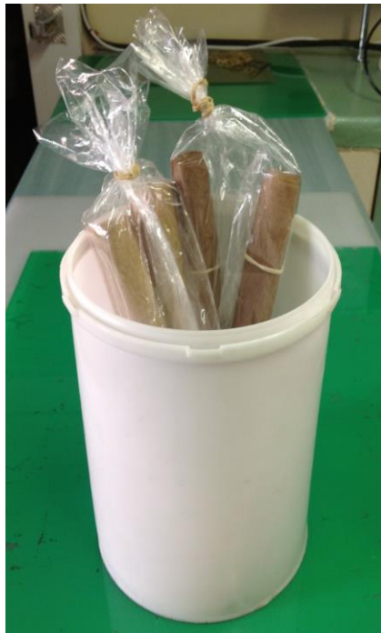
Figure 9: Four sheets of germination paper rolled up and placed in a plastic bag in an upright position for the between-paper germination method.
