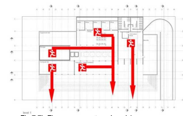
Fig 7.7b Fire escape routes - Level 1
