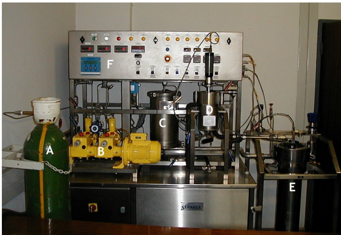
Figure 3.1: A 1ℓ PGSS reactor (Separex Equipments, France) used for encapsulation of bacteria, situated at the Polymers and Ceramics centre, CSIR, Brummeria, PTA. A= CO 2 supply, B= Pump, C= CO 2 preheater, D= Mixing chamber, E= Product chamber, F= Control panel
