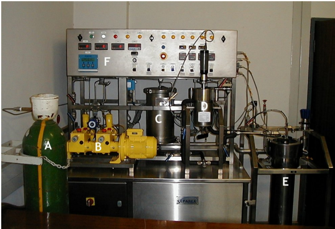
Figure 3.1: A 1ℓ PGSS reactor (Separex Equipments, France) used for encapsulation of bacteria, situated at the Polymers and Ceramics centre, CSIR, Brummeria, PTA. A= CO 2 supply, B= Pump, C= CO 2 preheater, D= Mixing chamber, E= Product chamber, F= Control panel
