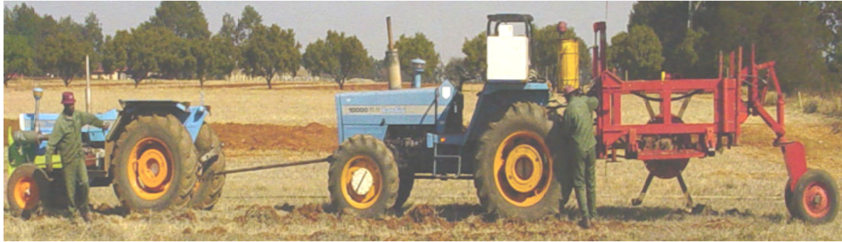
Figure 4.17: Setting-up for a tillage test-run [the swivel wheel at the rear end of the rotavator tool-frame carrier was lifted off the ground during tillage experiments]
