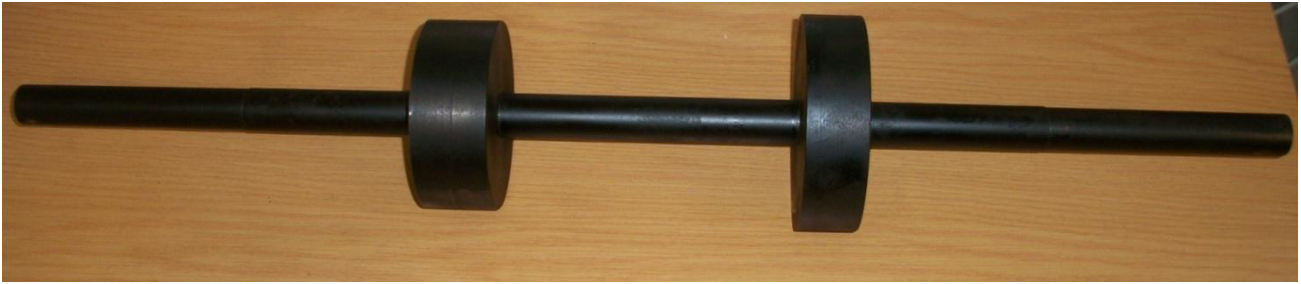
Figure 39 Manufactured rotor used for testing
