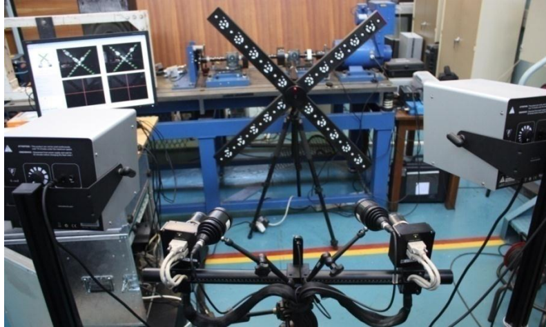
Figure 57 Calibration setup, calibration cross and strobe light positions
