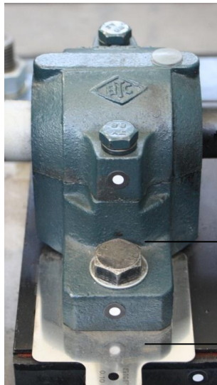
Figure 43 Bearing and spacer setup
