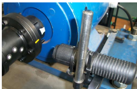
Figure 62 Tachometer setup with reflective tape
