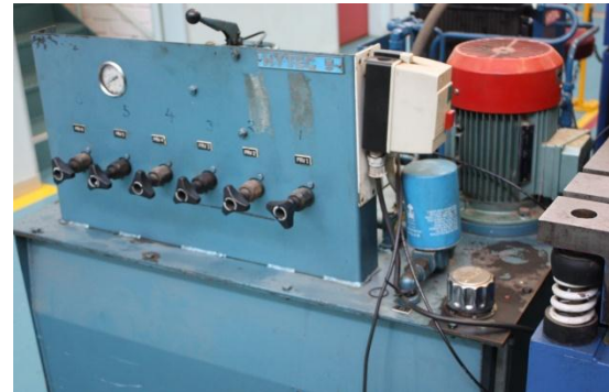
Figure 44 Pump for hydraulic brake
