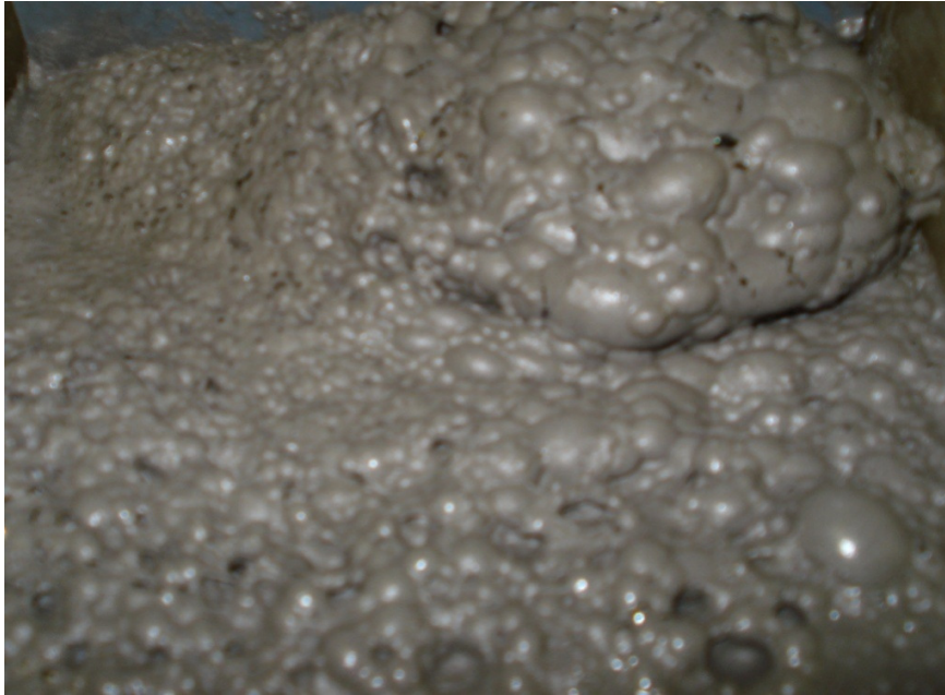
Figure 6.3: PCB CF froth in the flotation cell under natural hydrophobic response
