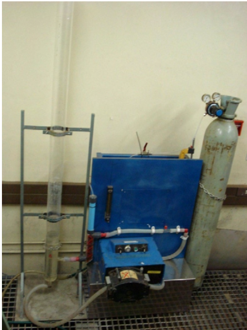
Figure A1.6: Betachem Modified Bikerman froth stability test rig
