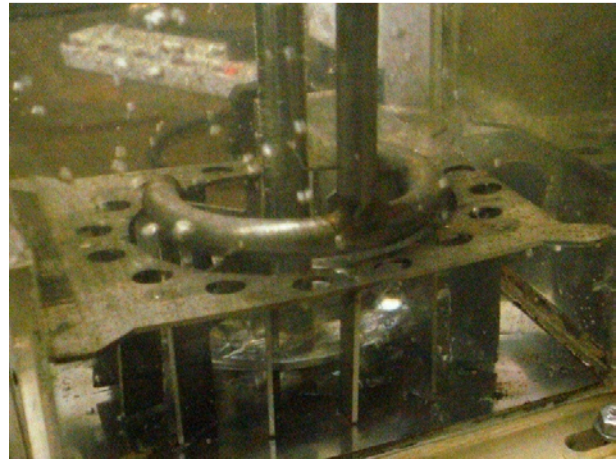
Figure A2.7: Frozen frames showing bubble sizes at 300 rpm impeller speed and 500 aeration rate (a) before and (b) after modification of the Leeds cell impeller system.
