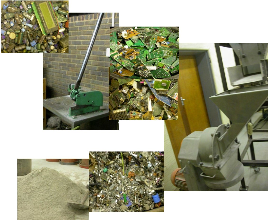
Figure A1.2: Pictorial flow of the comminution stages:
