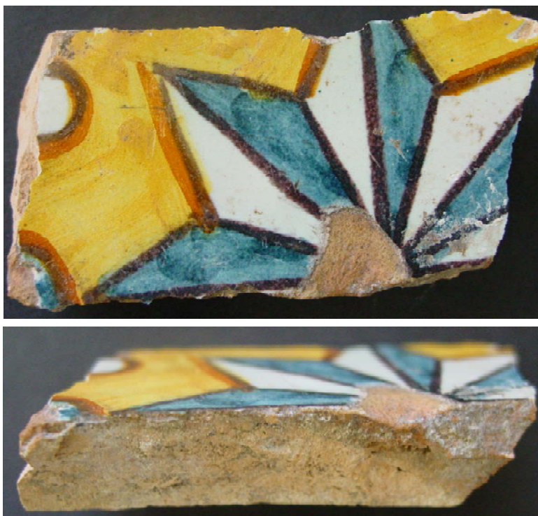
Figure 5.1.1. The different views of the Citadel tile highlight the different colours (above) and the relative thickness of the tile body (below) with respect to the glaze thickness
