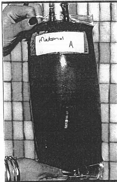
Plate 1. The anaerobic bioreactor (the expansion of the bag indicates gas production under anaerobic conditions).
