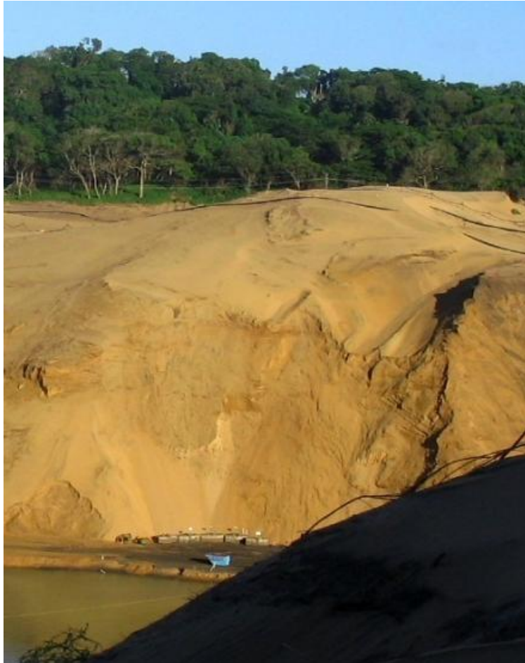
Plate 1-1. Mining operations at Richards Bay Minerals result in the removal of all vegetation and topsoil in front of the mining pond. Topsoil is stockpiled for use on rehabilitating sites. Immediately post-mining sand is formulated to an approximation of the dunes previous topography. The photograph was taken by Prof. R.J. van Aarde and is used with his permission.
