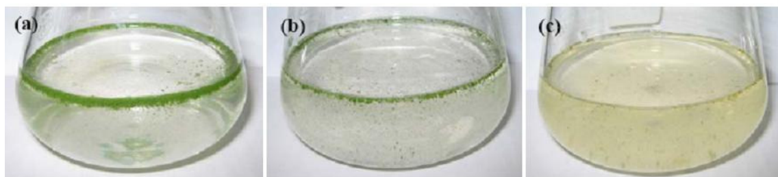
Figure 4: Cultures for re-growth experiment immediately after inoculation with cyanobacteria taken from the bottom of the beakers 36h after flocculation (a) inoculated with untreated cyanobacteria (Control); (b) inoculated with cyanobacteria treated with fly ash sample 5; (c) inoculated with cyanobacteria treated with fly ash 6.
