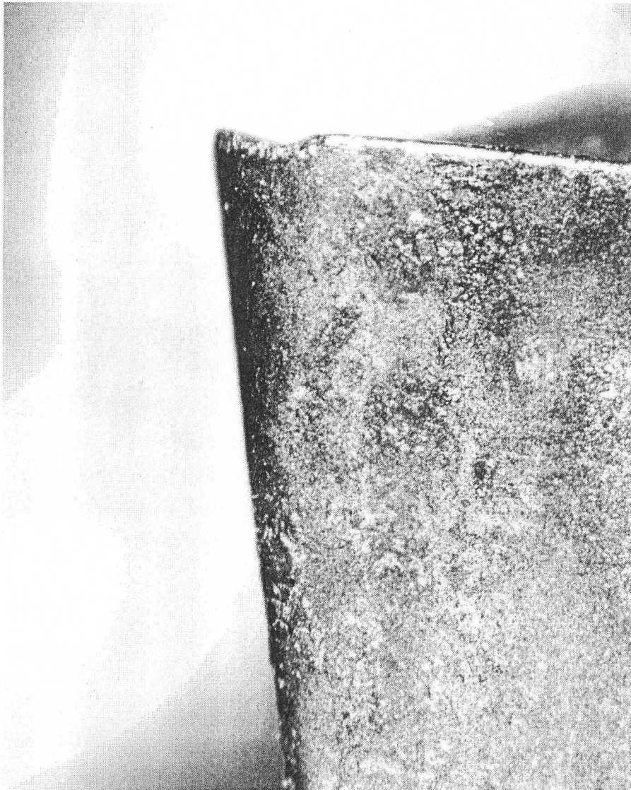
Figure C.3: Nose of a tool where wear has started
