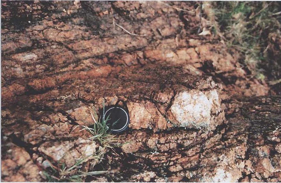
Figure 7.3: Crush breccia showing intense intrusion of quartz veins, which strike parallel to the strike of the southern strand of the Melinda Fault. Recorded at 23°07.39'S; 28°57.46'E. Lens cap is 5cm wide.
