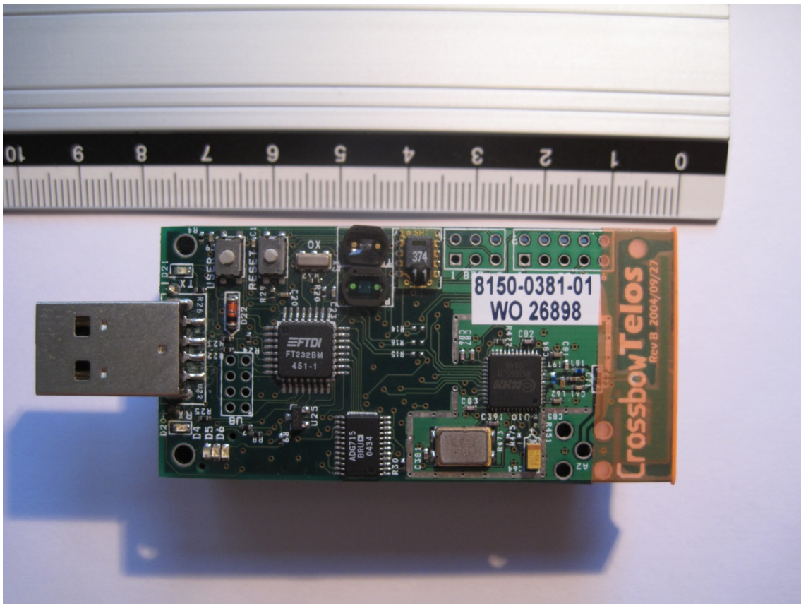
Figure 7.6. TPR2420 TelosB mote
