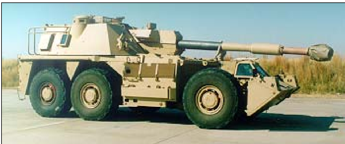
Figure 1-7: GV6 self-propelled howitzer fitted with semi-active rotary dampers
