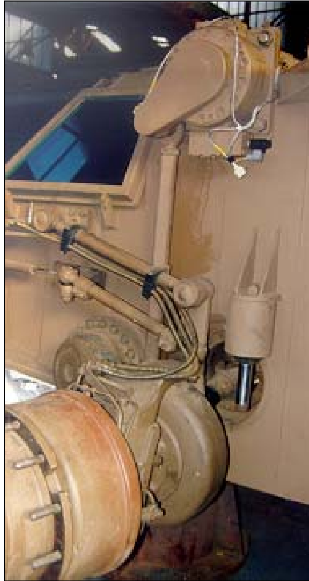
Figure 1-8: Semi-active rotary damper fitted to the experimental vehicle
