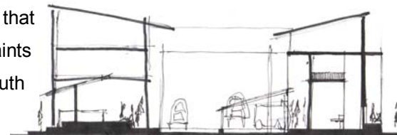
Figure 63 conceptual section and elevation illustrating vehicular access
