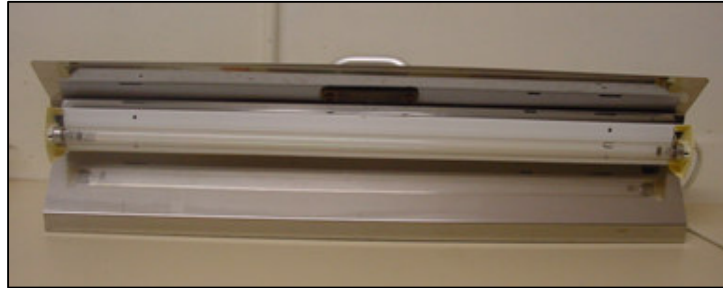
Fig. 3.1 Ultraviolet radiation light tube (Philips TUV 30W/ G30T8, 254 nm, in a fitting with a reflective aluminium backing) used to irradiate the eggs of three moth species ( Helicoverpa armigera , Chilo partellus and Cadra cautella ).
