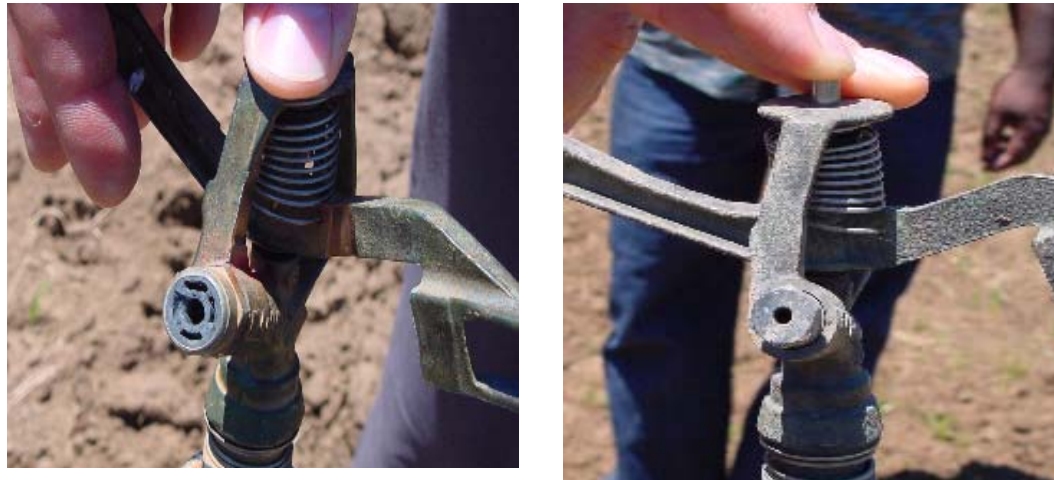
Photo 11. 2: Different sprinkler nozzles (a) CDS and (b) ordinary in use by a farmer in Zanyokwe (2004)
