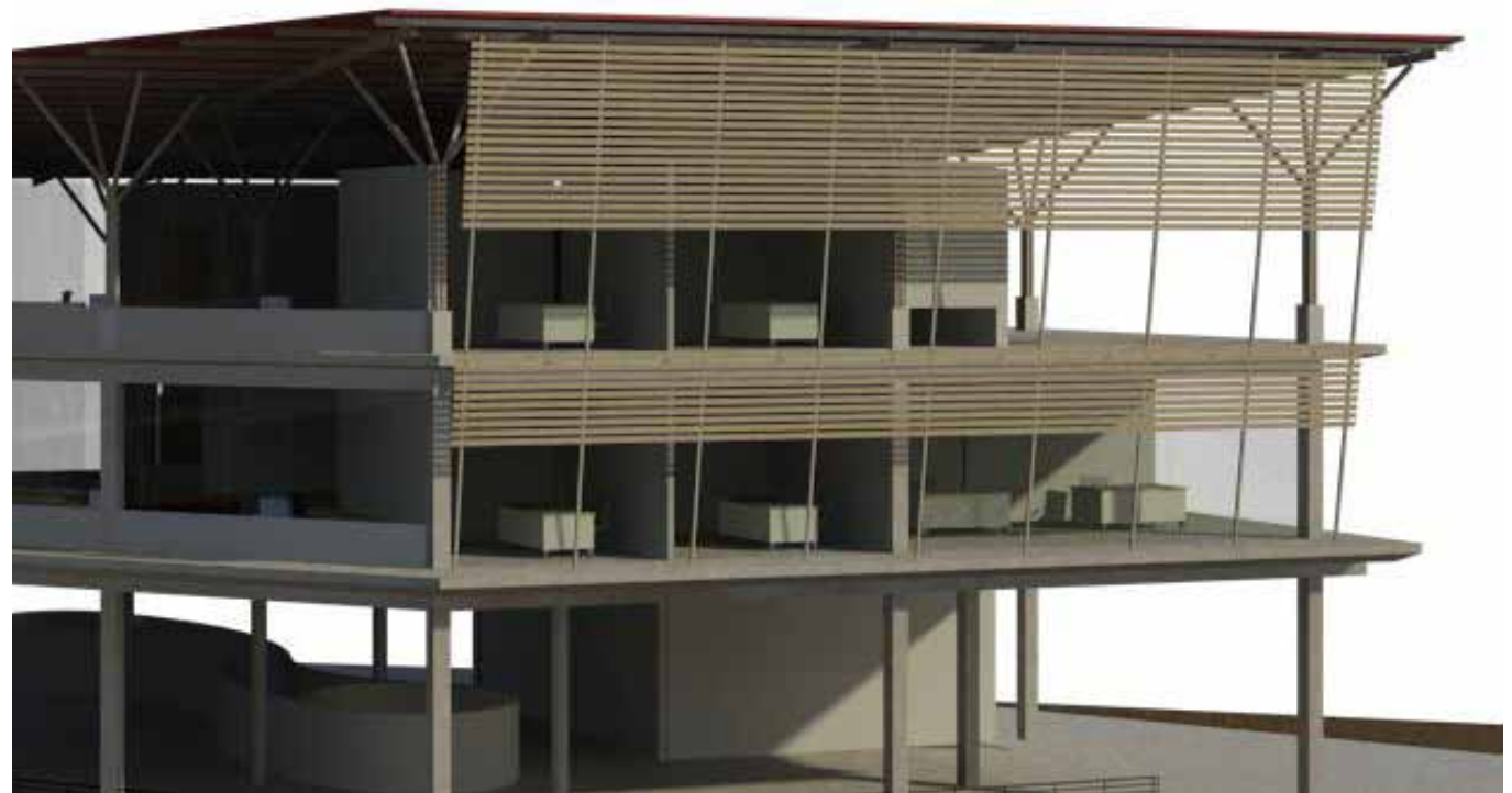
figure 152. 3d showing ecowood louvres on facade
