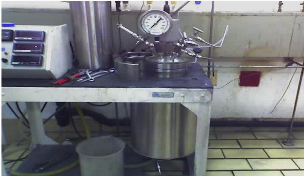
Figure 5.1 The 5 ℓ jacketed, pressurised & continuously stirred reactor used in CaS stripping experiments.
