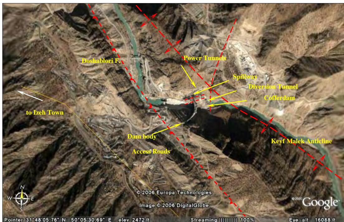
Figure 4.2.1. The satellite image of Karun-3 dam project and surrounding area before reservoir impoundment. This project located at 28 km east of Izeh town in Khuzestan Province. Access road of Dehdez – Izeh can be seen on middle part of picture (Google Earth, European Technology, 2009).
