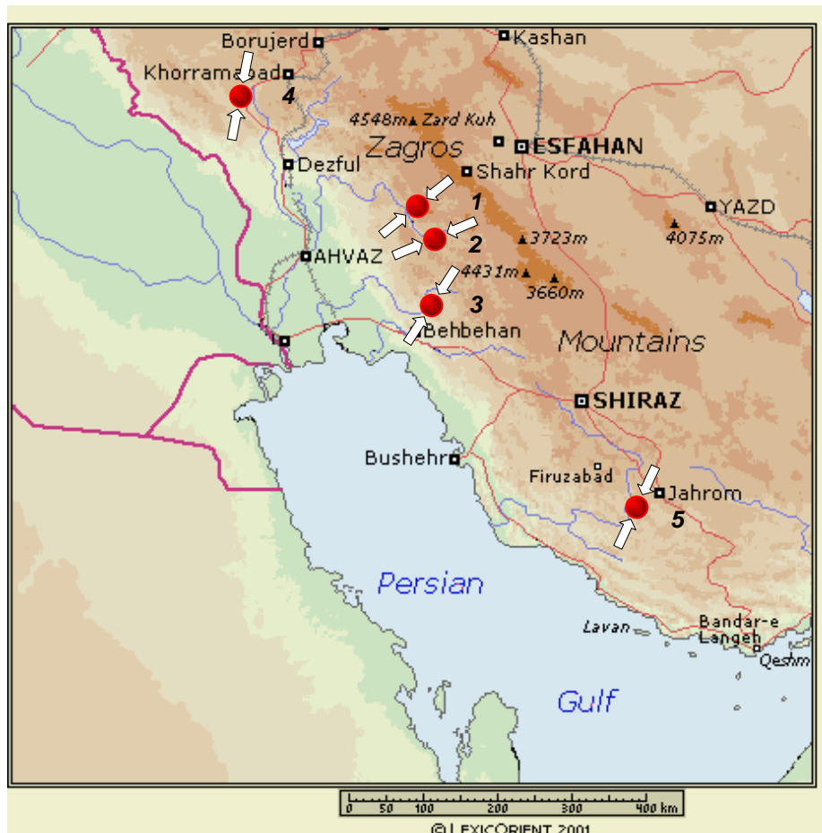
Figure 4.1. The topographical map of Zagros folded belt and locations of five dam sites. Seymareh (4), Karun-3 (1), Karun-4 (2), Marun (3) and Salman Farsi (5). The direction of shortening at the region due to tectonic movements are indicated by white arrows. (Lexicorient base map, 2001).
