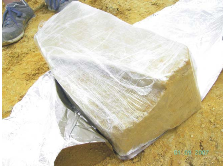
Figure 3-4. Wrapping the block sample to prevent moisture loss.
