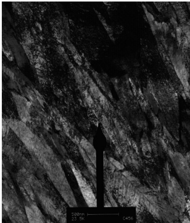
Figure 6.12(a): TEM selected area bright field of the steel H ( M_s = 210^\circ\text{C} )
