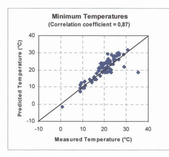
Figure 3.5 - Comparison between measured and predicted minimum temperatures for Test 1.
