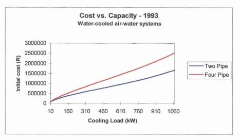
Figure 6.17 - Cost versus capacity relation for water-cooled air-water systems
