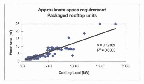
Figure 6.6 - Space requirement correlation for rooftop packaged units
