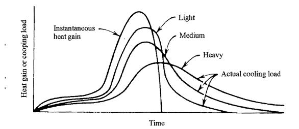
Figure 7.4 - Effect of thermal mass on HVAC system size [3].
