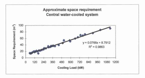
Figure 6.2 - Space requirement correlation for water-cooled all-air systems
