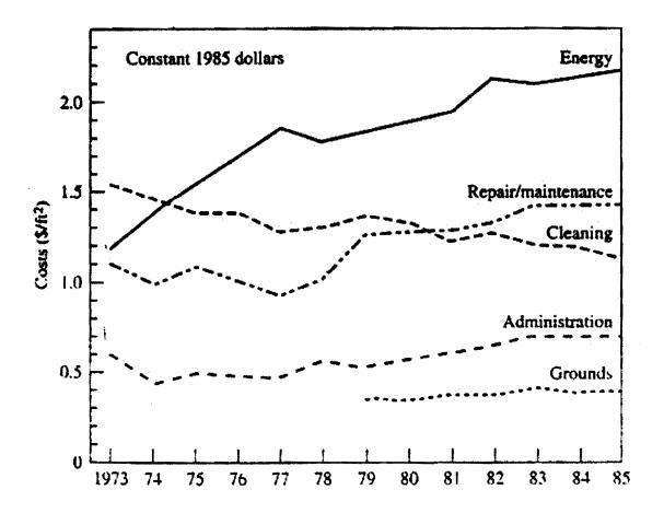
Figure 1.1 – Average office building operating cost per floor area corrected for inflation  $\frac{1}{ft^2} = 10.76/m^2$  [5]
