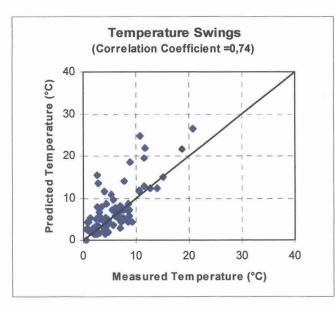
Figure 3.7 - Comparison between measured and predicted temperature swings for Test 1.
