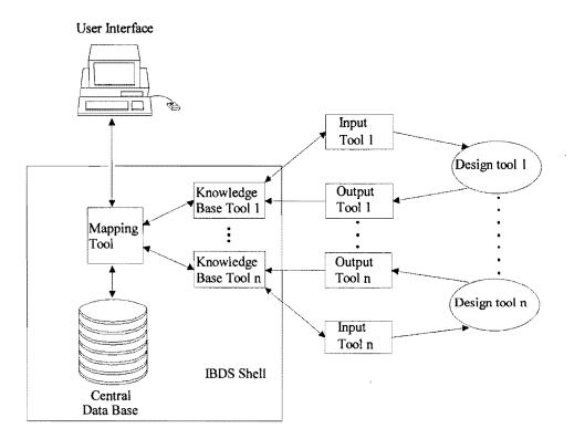
Figure 1.3 – Typical IBDS structure (Adapted from [13])
