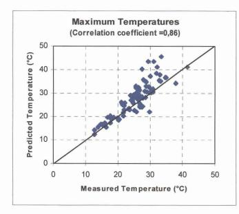
Figure 3.3 - Comparison between measured and predicted maximum temperatures for Test 1.
