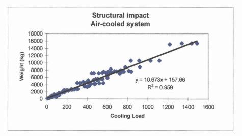
Figure 6.8 – Mass correlation for air-cooled refrigeration machine
