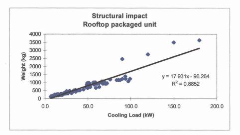
Figure 6.10 – Mass correlation for rooftop packaged units
