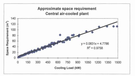
Figure 6.1 - Space requirement correlation for air-cooled all-air systems.
