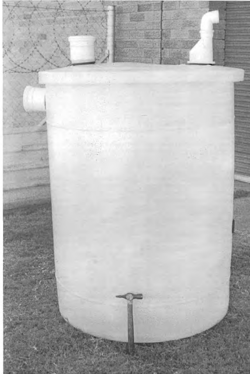
(e) The complete tank, fully assembled
