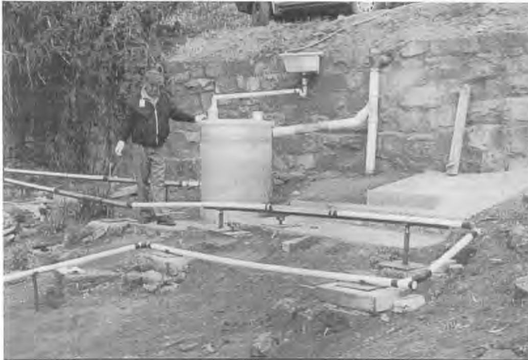
Figure 6.25: Experimentation with inverse pipe gradients
