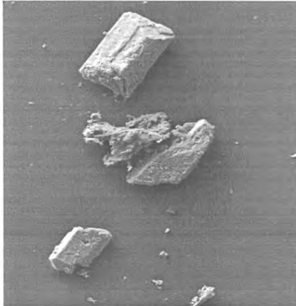
(a) Crystalline, white flakes: Main constituents: P, Mg, Ca (Magnification 59X)
