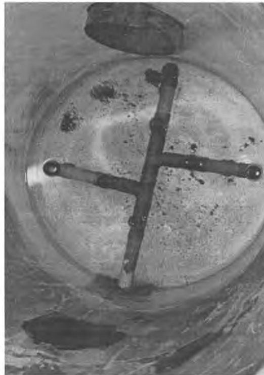
Figure 6.5: Multiple siphonic intake for withdrawing settled sawdust from tank (a) schematic illustration; (b) photograph of manifold inside tank
