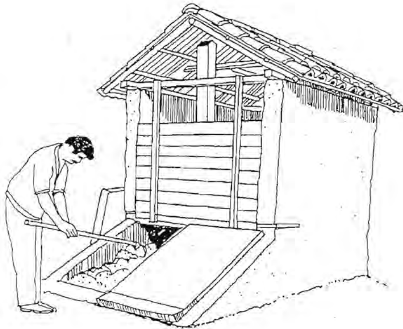
Figure 8.5: A solar-heated dehydrating toilet in Ecuador (Winblad 1996b)
