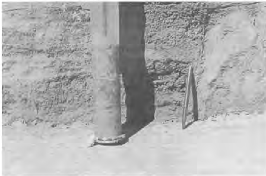
Figure 6.24: Typical sludge sample cored from the tank before testing of the system (the core represents the sludge accumulated above the level of the grille).
