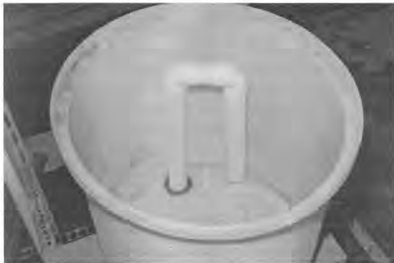
Figure 6.1: 50 l container and 50 mm diameter prefabricated pipe system intended to simulate a siphonic-type outlet
