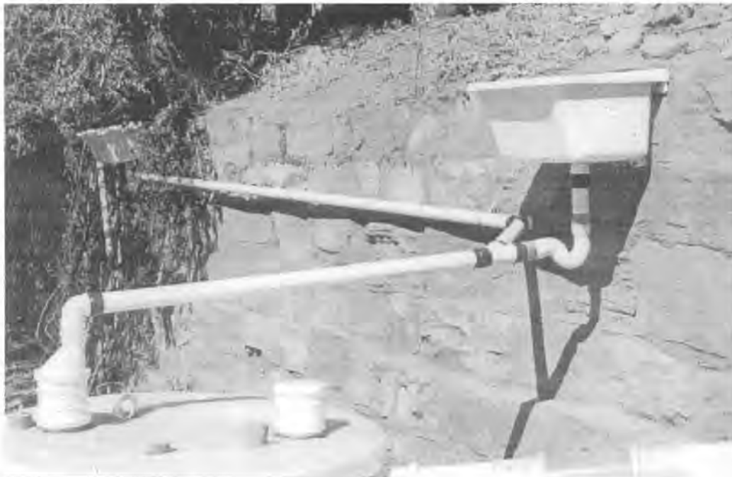
Figure 6.26: Testing the effect of different wastewater flow distances on the operation of the siphon.
