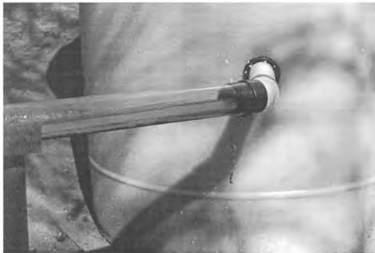
(f) Flow emerging from tank before activation of flush (i.e. normal overflow from influent)
