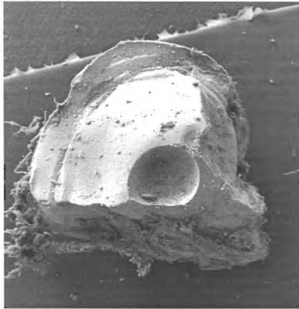
(c) Shiny black particle: Main constituents: Fe, Si, Ca, Mn, K, Cr, S, Al (Magnification 43X)
