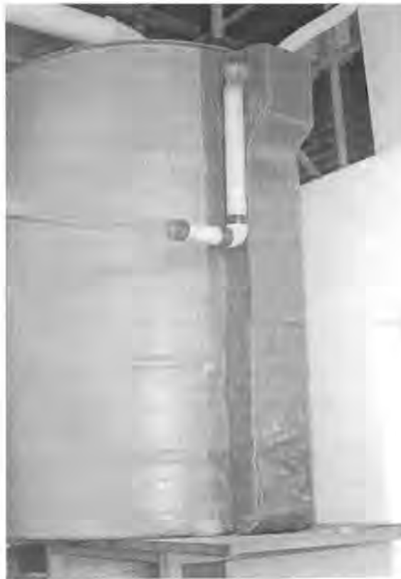
Figure 6.15: Apparatus set up to produce a discharge head of 0,5 m
