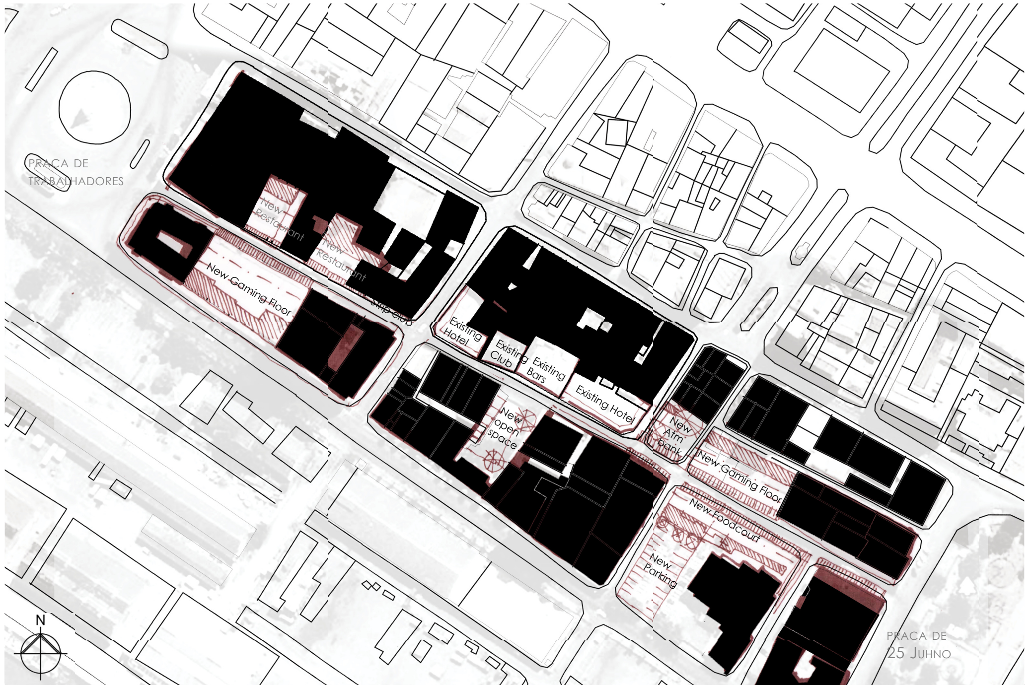
Figure 5.54 plan showing all new functions interspersed with the existing, superimposed on a noll-type map showing precinct inclusive spaces in white and non-precinct functions in black.
