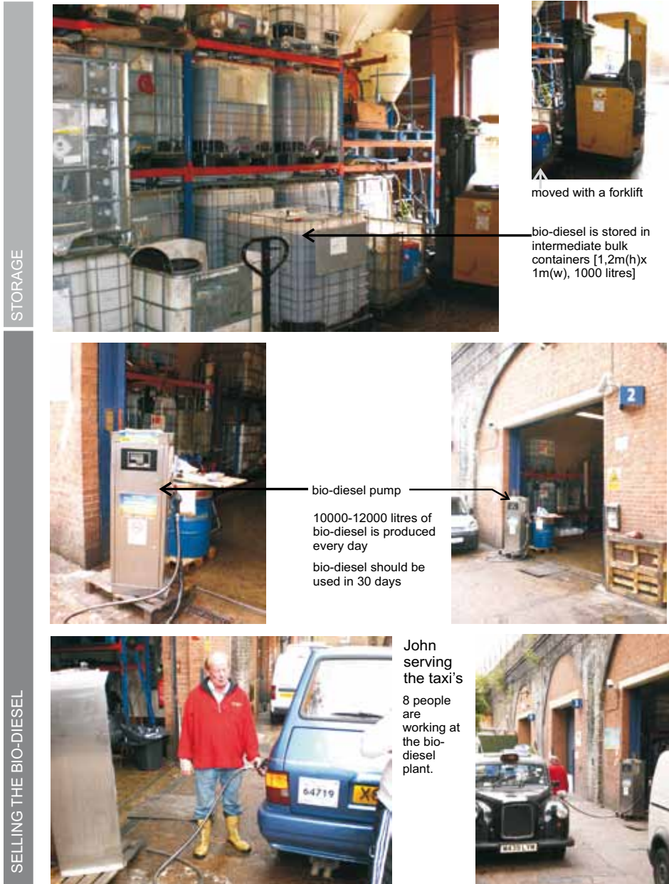
Figure 70. Diagram showing the production process of bio-diesel at Uptown oil, London, UK. Photographs by author (visited in June 2010).
