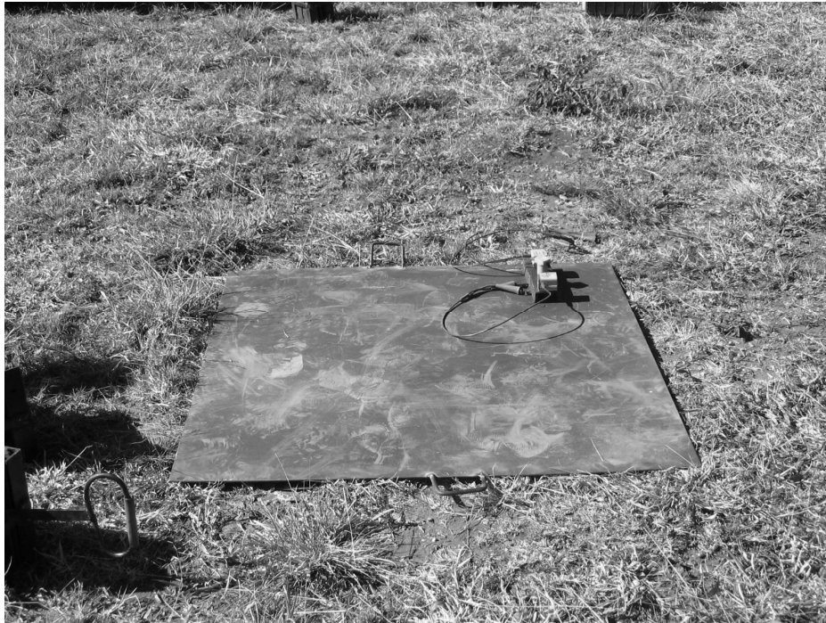
Fig. 1. Large bearing plate with geophones mounted for measurements in three directions.
