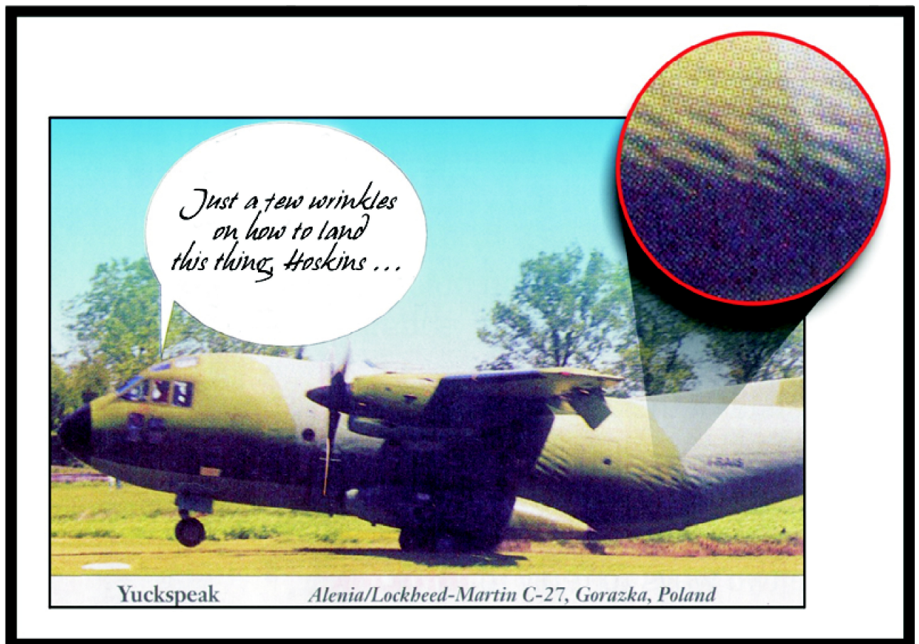
Figure 1: An illustrative example of shear buckling (Reproduced from Flight International , 8-14 September, 1999)
