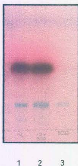
Figure 6.4: TLC on a glass plate of fraction 12 (1) of the acetone extract of H. hemerocallidea that eluted from the first column with ethylacetate:methanol:water (10:1.35:1) as mobile phase. Co-chromatographed is fraction 12 spiked with \beta -sitosterolin (2), and isolated \beta -sitosterolin (3). The plate was developed in CEF and sprayed with p -anisaldehyde.
