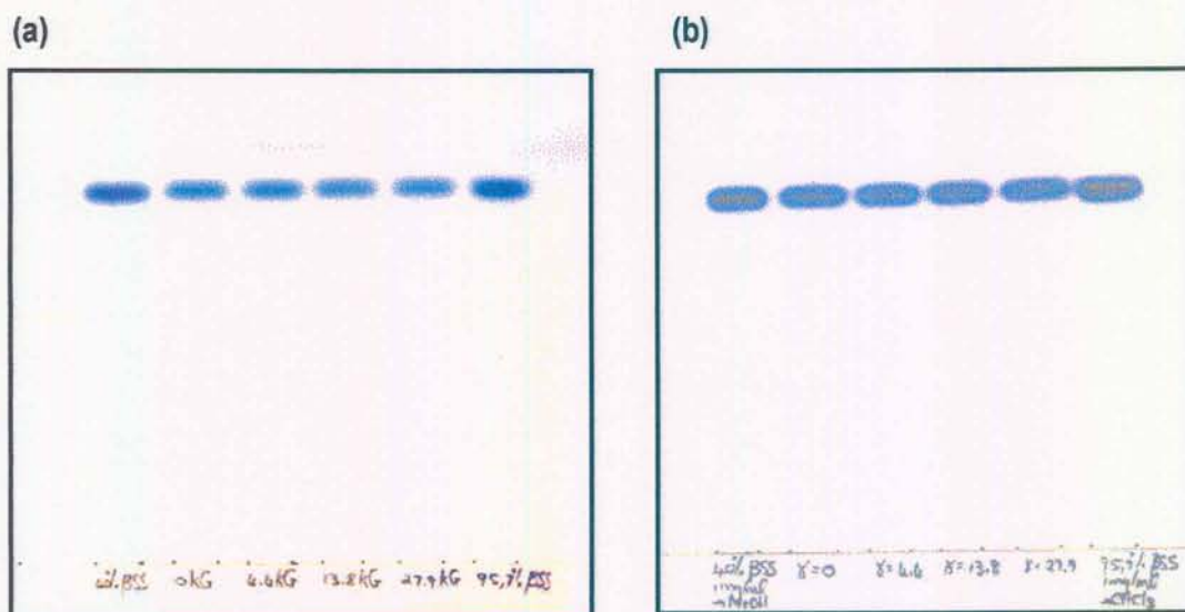
Figure 5.12: TLC on aluminium plates of chloroform extracts of (a) Immunochoice ® and (b) Moducare ® , gamma irradiated at 0, 4.4, 13.8 and 27.9 kGray. On the sides are 40% \beta -sitosterol standard.
