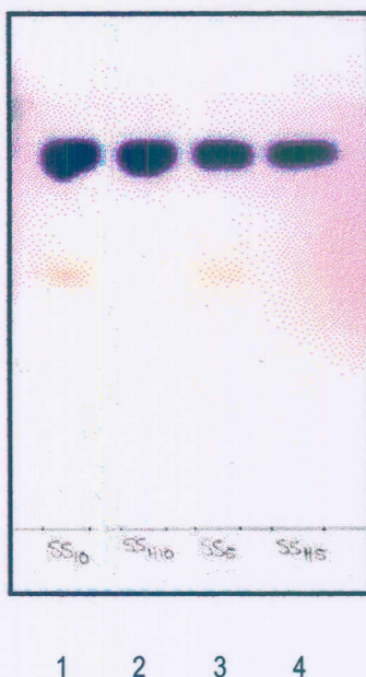
Figure 3.8: Overheated TLC on a glass plate of unhydrolysed (1) and hydrolysed 10 mg/ml 95% stigmasterol standard (2) and unhydrolysed (3) and hydrolysed 5 mg/ml 95% stigmasterol standard (4).
