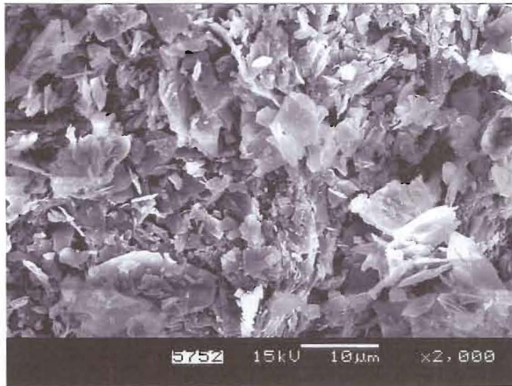
Figure 3-65: Pay Dam Penstock Coarse Tailings, undispersed bulk specimen.
