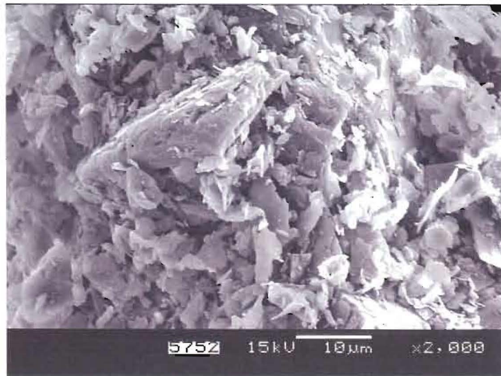
Figure 3-62: Mizpah Pond Fine Tailings, undispersed bulk specimen.
