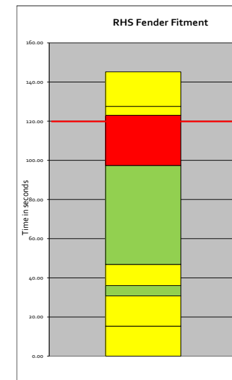
FIGURE 21: YAMAZUMI CHARTS OF RHS FENDER FITMENT STATION UNDER ABNORMAL CONDITIONS
