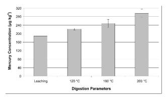
**Figure 2.** Mean mercury concentrations determined in lichen stock aliquots subjected to different digestion temperatures (n=3), where error bars depict the standard deviation. In all cases 1 mL of nitric acid was used. The leaching experiment was conducted at room temperature, whilst the other temperatures were obtained by microwave heating.
