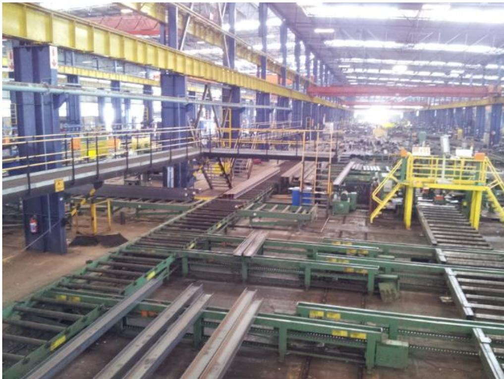
Figure 19: Automated roller conveyor system
