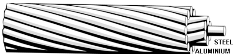
Figure 8: The basic make-up of an ACSR conductor.
