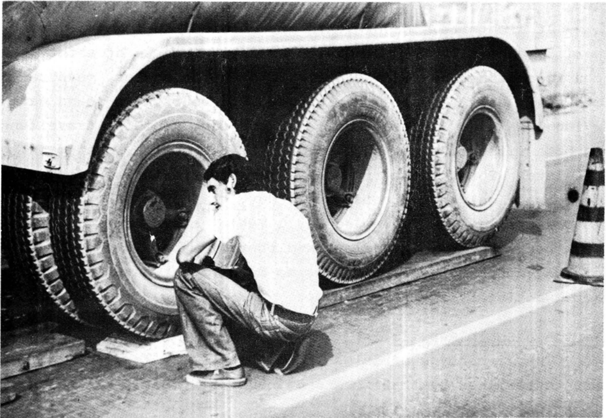
Figure 29 - Axle Weighing with Portable Scales
