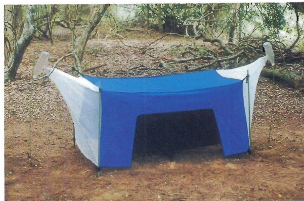
FIG. 2 Photograph of the final H trap design for the live capture of G. brevipalpis and G. austeni (the trap is held upright by fastening the corners to four rigid metal poles (1,2 m long) and the cones are suspended from two flexible steel rods (1,4 m)
