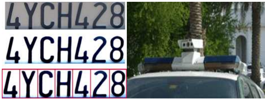
Picture 11: Optical Character recognition preparation and camera.
